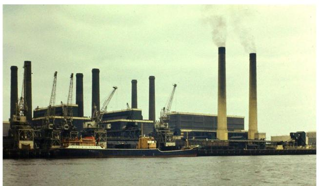
The ship is the CEGB collier Sir Archibald Page. Powered by a triple-expansion steam engine she was built at Sunderland in 1950. Sold abroad in 1972 the vessel was broken up in March 1980.
