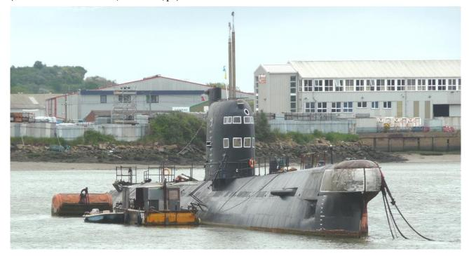
Now in a bad external condition one side of the hull is being repainted, the other side is red with rust and red oxide so remedial work is being undertaken there. But it is of course a massive task and moreover this painting is only taking place above the waterline, expensive dry docking would be required to preserve the rest of the hull. It was reported that the interior of the submarine is still in quite good condition. Does anyone have up-to-date information? *Bob Carr*
